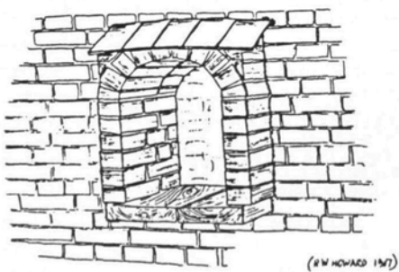
A pair of bee boles at Yew Trees House, Boxley (90). The slots above show where the tiled roof was once fixed, as suggested by the drawing. (Photo. and drawing: R.W. Howard, 1987)
